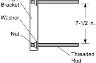
that the posts have to fit inside the mounting clamps (assuming you wish to use the hardware provided by Electro-Mech). The standard clamps form a "pocket" that is 7-1/2 inches square. So, if you try to use a 10-inch diameter pipe, our clamps will not work.
